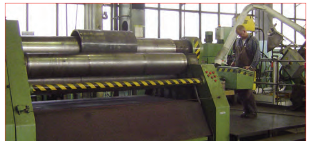
Plate rolling system for large diameter shells
