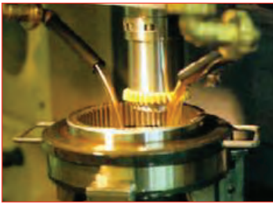
CNC gear shaping
